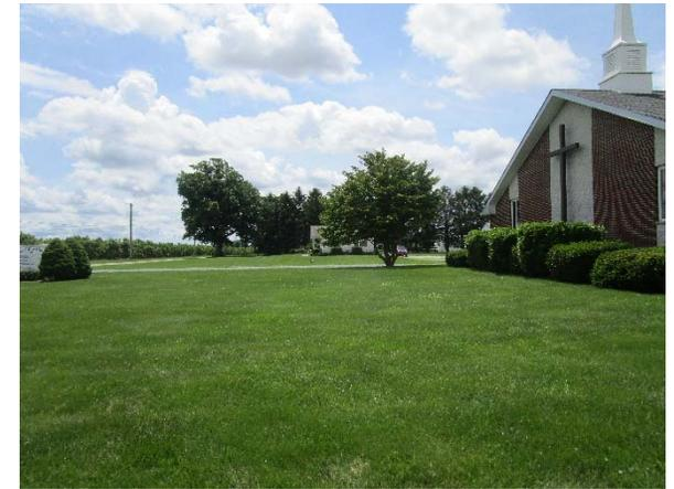
A rain garden can be installed in the turfgrass area between the church building and street, and a second can be installed along the north end of the building. The rain gardens will be able to capture runoff from the roof of the church by directing the downspouts to the gardens while also providing aesthetic value. A preliminary soil assessment suggests that the soils have suitable drainage characteristics for green infrastructure.
