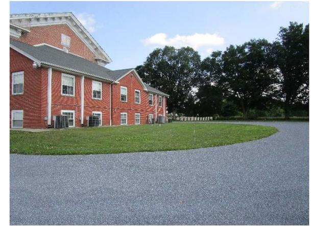
Three rain gardens can be installed in the grassed area adjacent to the church building to capture runoff from the roof of the building. Pervious pavement can also be installed in the parking spaces at the back of the building to capture and treat runoff from the surrounding pavement. A preliminary soil assessment suggests that the soils have suitable drainage characteristics for green infrastructure.
