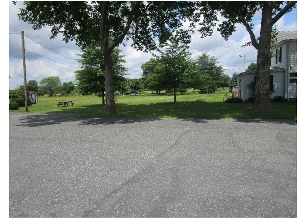
Pervious pavement can be installed north of the church building over the strip of asphalt at the edge of the turfgrass. Stormwater runoff from the roof of the building as well as the surrounding asphalt can be captured and treated by the pervious pavement. A small rain garden can be installed near the west building to capture runoff from the building's rooftop. A preliminary soil assessment suggests that the soils have suitable drainage characteristics for green infrastructure.
