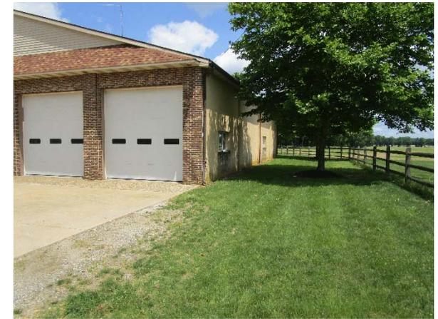
A cistern can be installed behind the building to capture and store stormwater runoff from the roof of the building that could be used to wash fire trucks or for other non-potable uses. A rain garden can additionally be installed along the southeast corner of the building by redirecting nearby downspouts into it. A preliminary soil assessment suggests that the soils have suitable drainage characteristics for green infrastructure.
